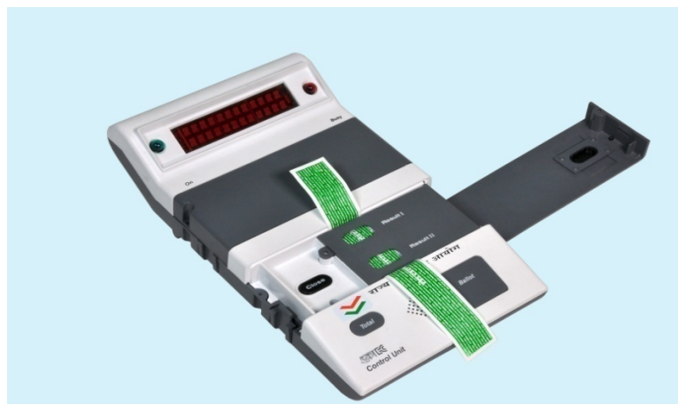
Fig. (b): CLOSING OF INNER COMPARTMENT WITH GREEN PAPER SEAL
