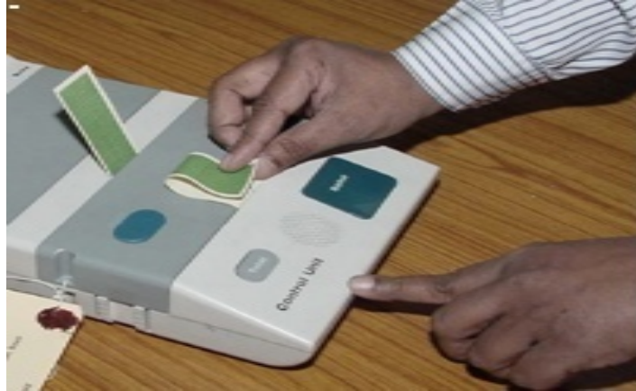
Fig. (d): SEALING PROCESS OF GREEN PAPER SEAL
